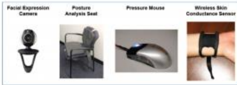
Exhibit 11. Four parallel streams of affective sensors used while a student is engaged in Wayang Outpost, an online tutoring system
